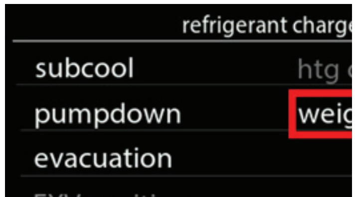
Fig. 16 – Weigh-in Option for charging below 65°F OAT and above 105°F OAT
