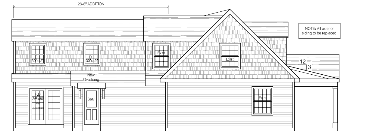
NORTH ELEVATION - SIDE
