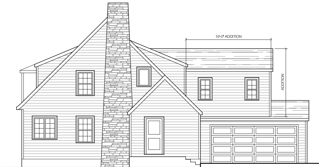
FRONT ELEVATION - Rear Addition w/ Hip Roof
