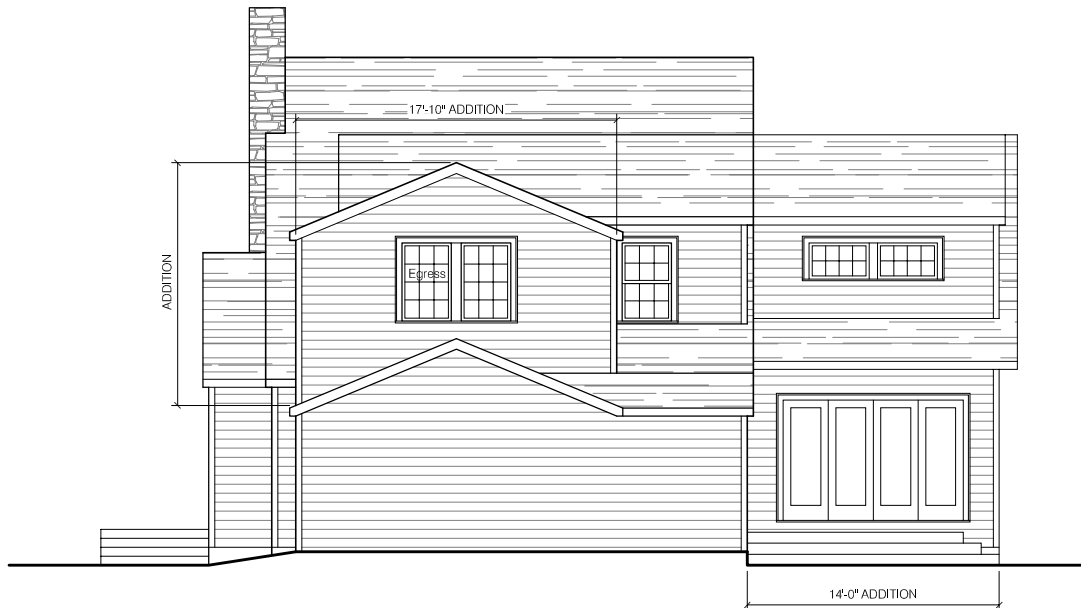
NORTH SIDE ELEVATION - Rear Addition w/ Gable Roof
