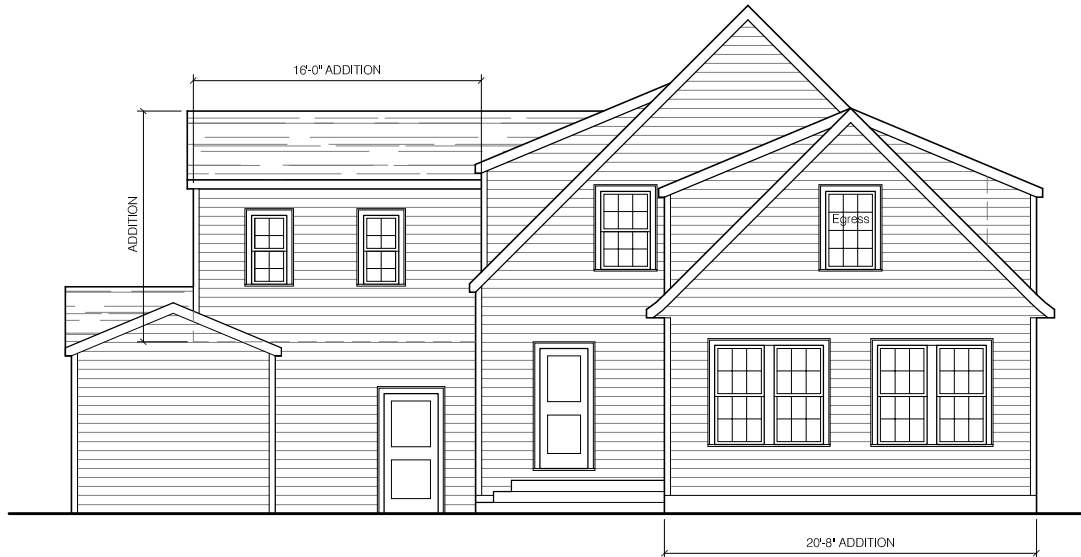
REAR ELEVATION - Rear Addition w/ Gable Roof
