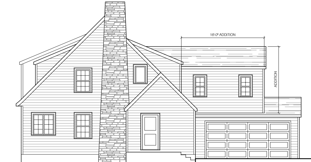
FRONT ELEVATION - Rear Addition w/ Gable Roof
