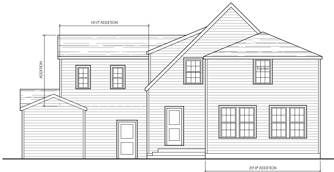
REAR ELEVATION - Rear Addition w/ Hip Roof
