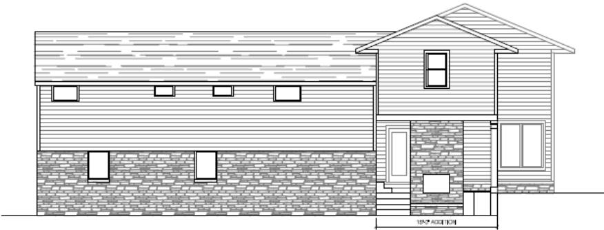
EAST ELEVATION (Side) - w/ Addition
