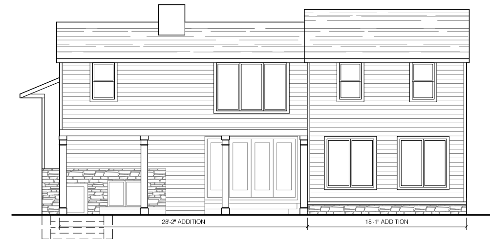
NORTH ELEVATION (Rear) - w/ Addition
