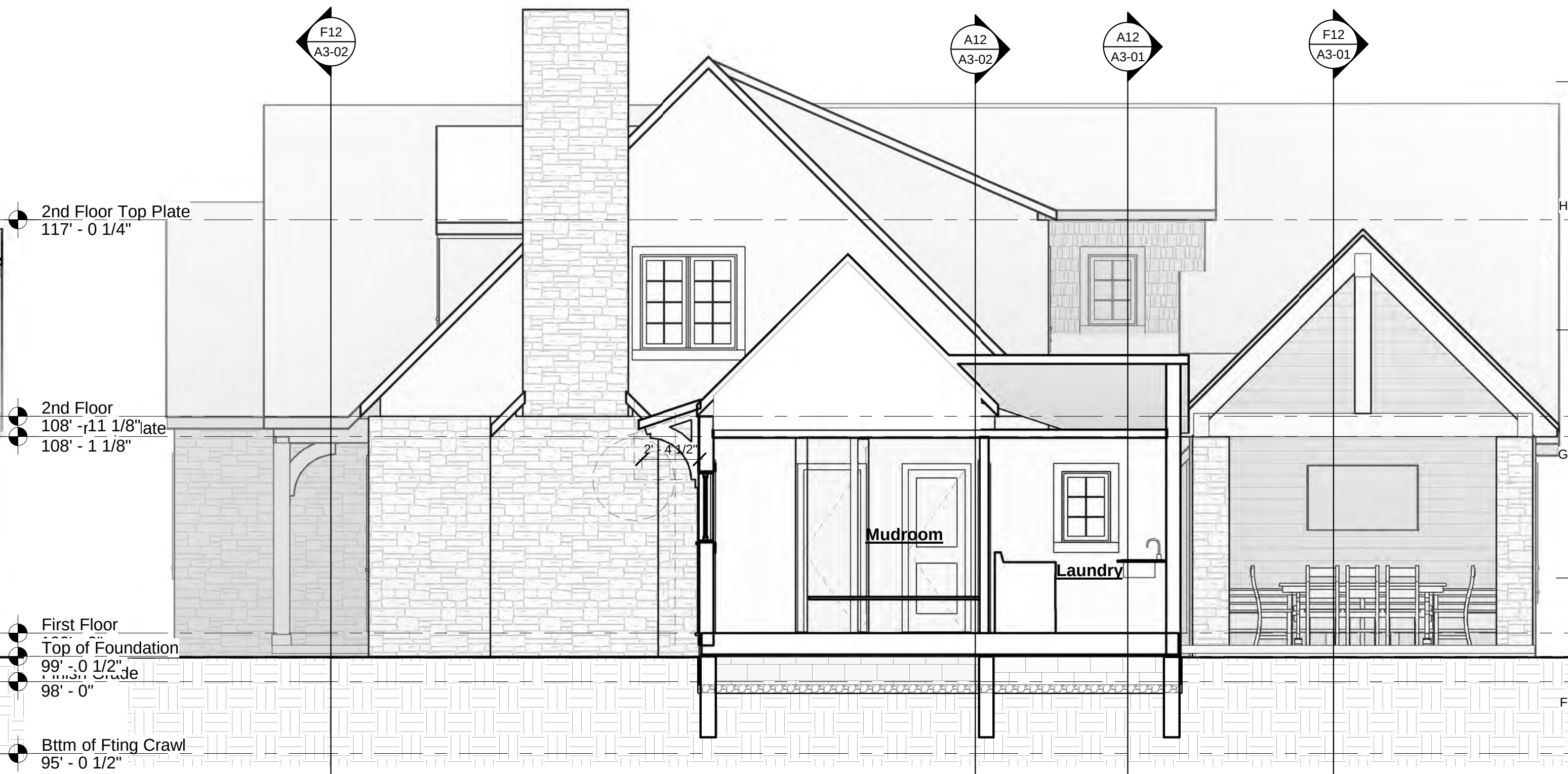
F6 Building Section - Infilled Connector 1/4" = 1'-0"
