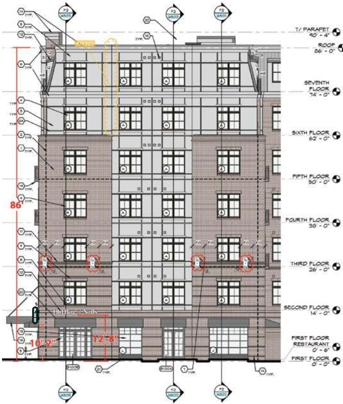
D2 SOUTHWEST PARTIAL ELEVATION 1/8" = 1'-0"
