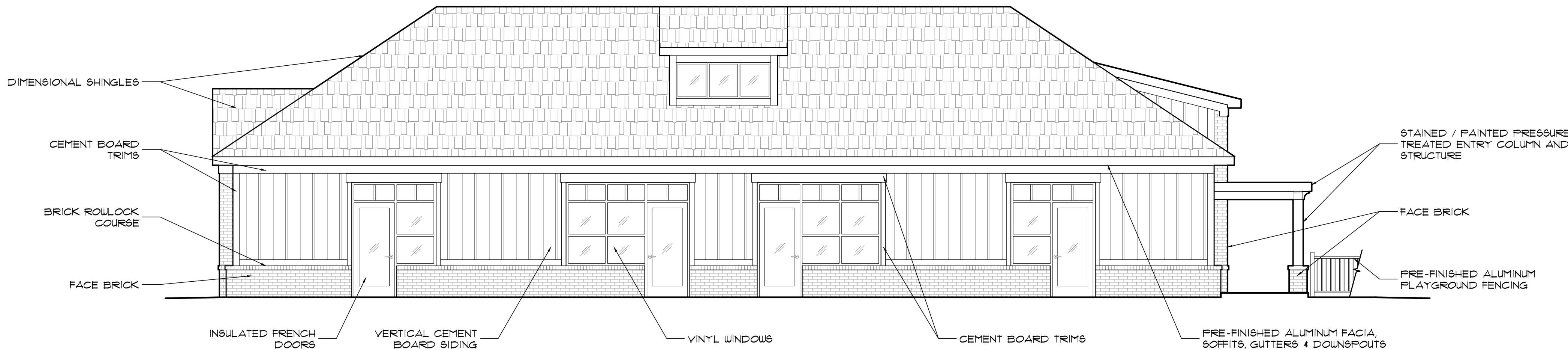
EAST ELEVATION - (DROP OFF)
