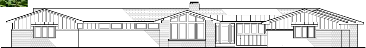
1 EAST ELEVATION - NEW WORK SCALE: 3/16" = 1'-0"
