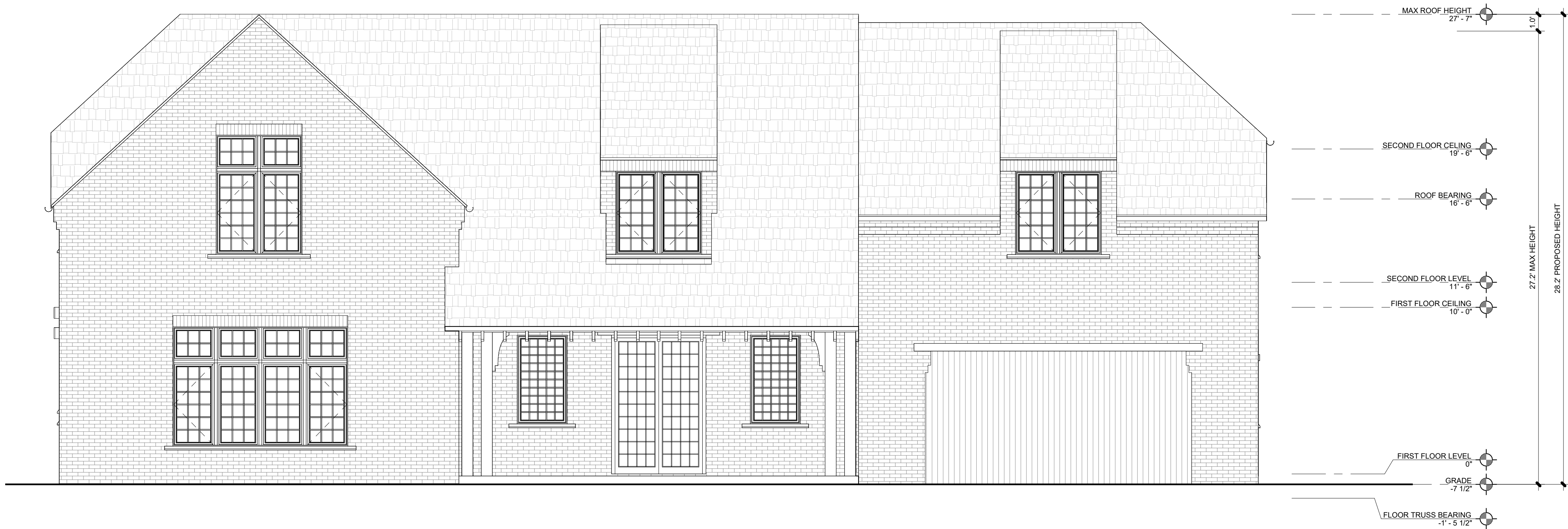
1 EXTERIOR ELEVATION - SOUTH FACING SCALE: 1/4" = 1'-0"
