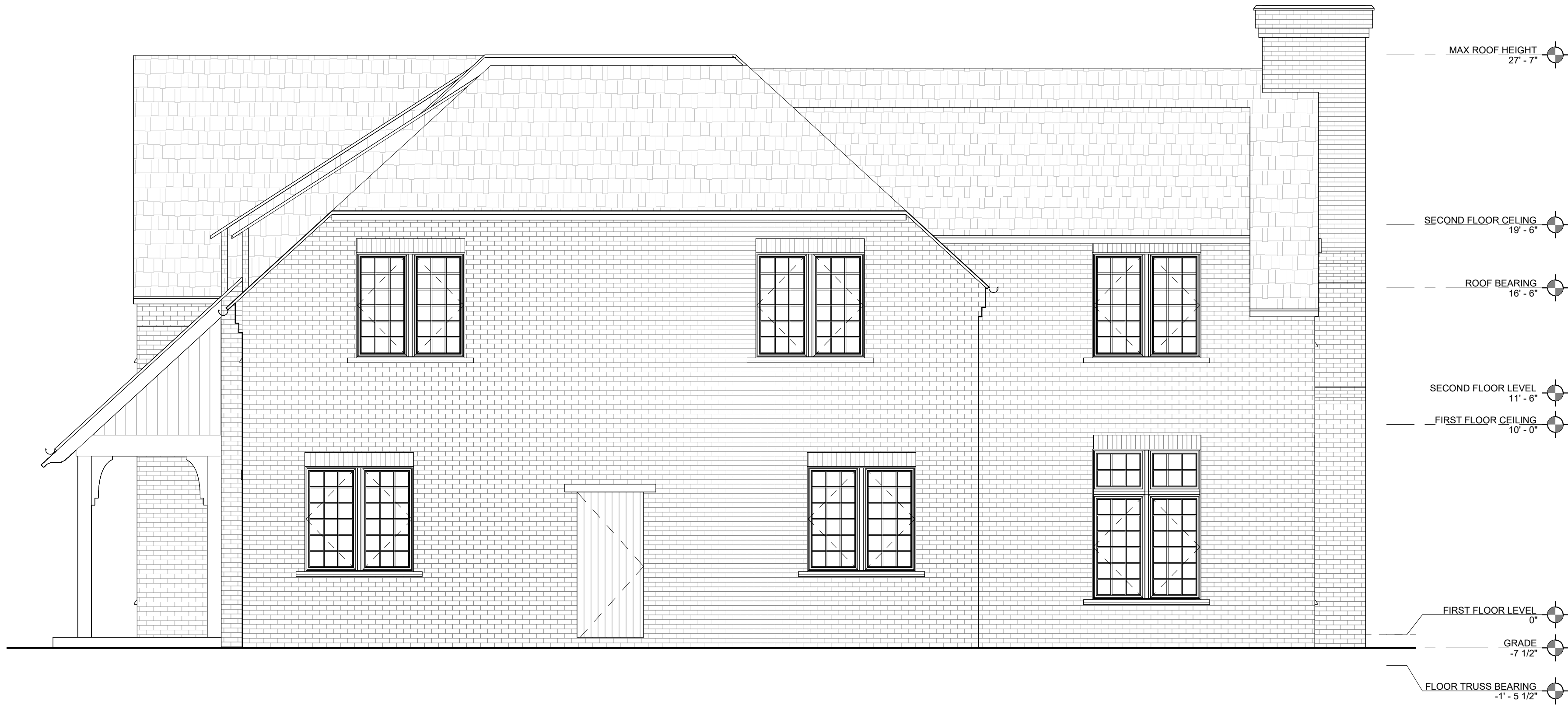
2 EXTERIOR ELEVATION - EAST FACING SCALE: 1/4" = 1'-0"
