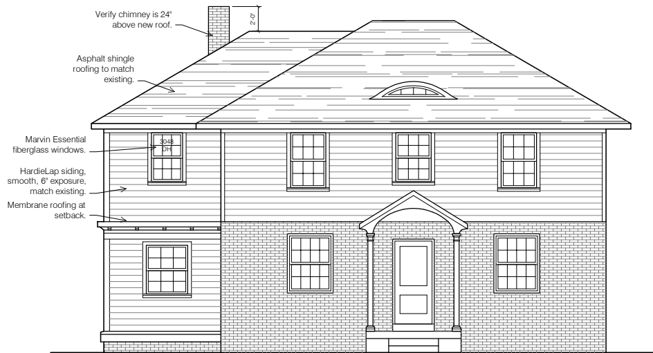
West Elevation - w/ Addition
