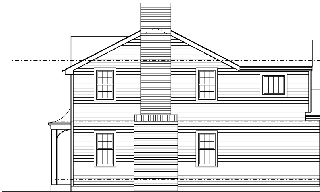
ASBUILT EAST ELEVATION
